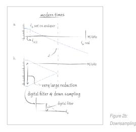
A consequence is however that we are left with a high-sampled signal of which only a small frequency range is of interest. So obviously, the signal needs to be down sampled to an order of magnitude of kHz.
