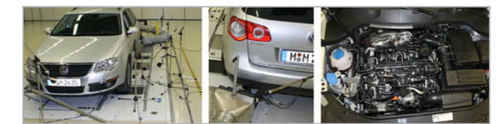
Figure 6: The measurement setup for the Contribution Analysis during the simulated pass-by measurement with microphones at intake, tires, exhaust, and inside the engine. Accelerometers on the engine and exhaust system provide additional valuable information for statistics
