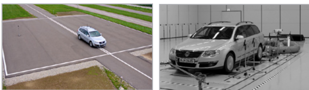
Figure 1: A test track for outdoor pass-by measurements on the left side. The setup for indoor pass-by on the right
