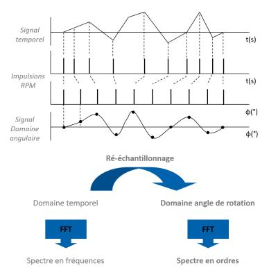
It allows to aply a FFT analysis with te sampling frquency and a time bloc adapted to the rotational speed.  $\Delta f$  increases with the rpm / the bloc duration dicreases when the reotational speed increases / the order resolution is constant
